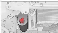
8. Use needle nose pliers to remove the desiccant bag from the accumulator.
