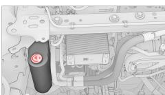
4. Hand-tighten the new dust cap to the accumulator.
