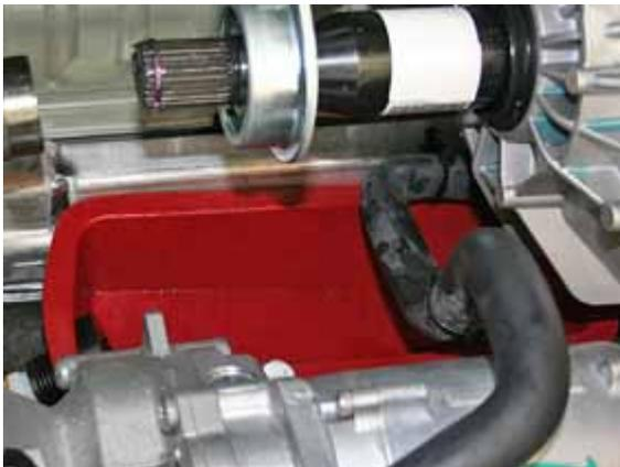
4. Remove the fill plug (torque 28 Nm).
