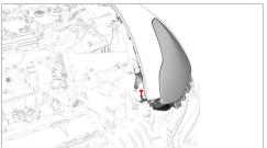
8. Remove the fastener(s) that attach the LH headlight to the body.
