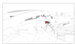
Connect the electrical connector for the LH headlight.
