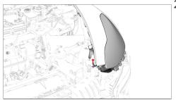
Install the fasteners that attach the LH headlight to the body.
