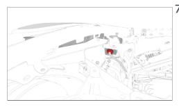
Disconnect the electrical connector from the LH headlight.
