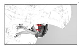
14. Remove the bolts that attach the LH front hub to the LH front knuckle.
