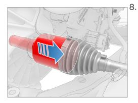
8. Pull on the inner halfshaft cup to confirm that the circlip is locked into place. If the halfshaft detaches from the drive unit then reinstall the halfshaft and then test that it is fully seated.
