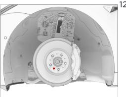
12. Remove the bolt that attaches the LH front brake rotor to the hub, but do not remove the rotor at this time.
