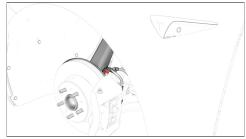
**11.** Remove and discard the bolts that attach the LH front brake caliper to the LH front knuckle, and then hang the caliper aside with an S-hook.
