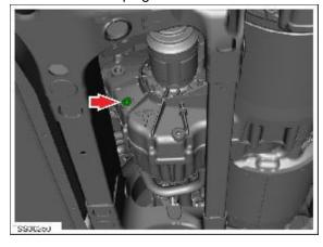
6. Remove the drain plug and allow the liquid to drain into the container.
